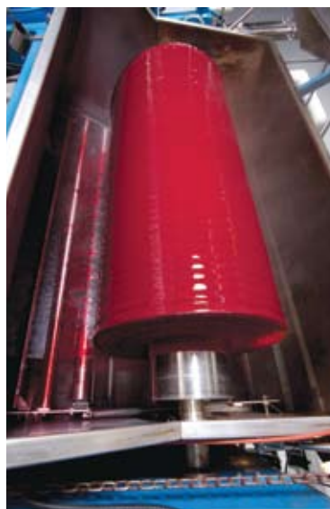
BELOW: A dye jig in South Boston. Annin has dyed its own nylon since 2007, making the flagmaking process more efficient.
